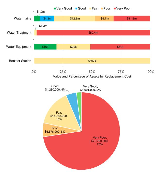
To ensure that the Town's water network continue to provide an acceptable level of service, the Town should monitor the average condition of all assets. If the average condition declines, staff should re-evaluate their lifecycle management strategy to determine what combination of maintenance, rehabilitation, and replacement activities is required to increase the overall condition of water network.
