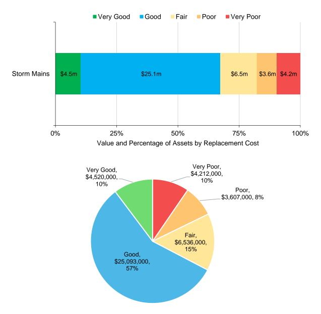
To ensure that the Town's storm network continue to provide an acceptable level of service, the Town should monitor the average condition of all assets. If the average condition declines, staff should re-evaluate their lifecycle management strategy to determine what combination of maintenance, rehabilitation, and replacement activities is required to increase the overall condition of the storm network.
