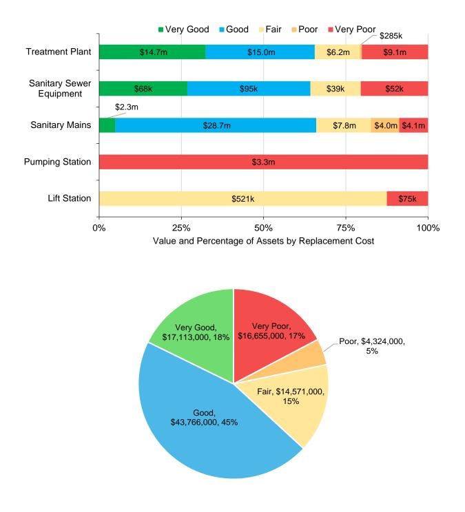
To ensure that the Town's sanitary sewer network continue to provide an acceptable level of service, the Town should monitor the average condition of all assets. If the average condition declines, staff should re-evaluate their lifecycle management strategy to determine what combination of maintenance, rehabilitation, and replacement activities is required to increase the overall condition of sanitary sewer network.
