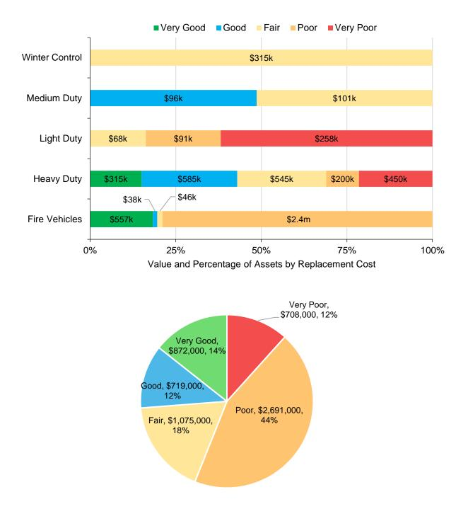
To ensure that the Town's vehicles continue to provide an acceptable level of service, the Town should monitor the average condition of all assets. If the average condition declines, staff should re-evaluate their lifecycle management strategy to determine what combination of maintenance, rehabilitation, and replacement activities is required to increase the overall condition of vehicles.
